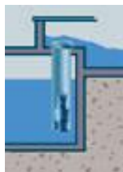
The basic design is the same as in previous illustration, but the pump is placed in a steel column that rests on a support frame.
