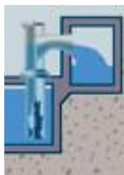
A closed system with either a free discharge, as shown, or with a flap valve.
