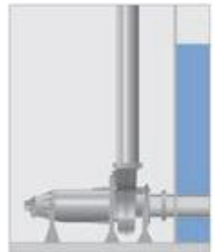
CZ – A horizontally-mounted, permanent dry well or in-line installation with flange connections for suction and discharge pipe work.
