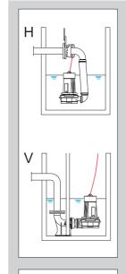
Pumps are available for permanent fixed installation, using the guide rail coupling V or the header coupling H, that is installed above the water level.
