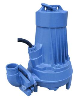
The RS2210 series is limited in flow to just over 4 l/s  $(15 \text{ m}^3/\text{h})$ . With this flow the flow velocities are sufficient in discharge pipes with 80 mm bore or less. It is recommended not to select duty points on the vertical part of the QH-curves. Short term running on these sections is allowed.
