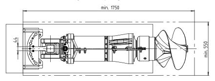
L<sub>1</sub> should be located as closely above the mixer as possible to ensure that the forces generated are safely transferred from the guide rail to the wall!
