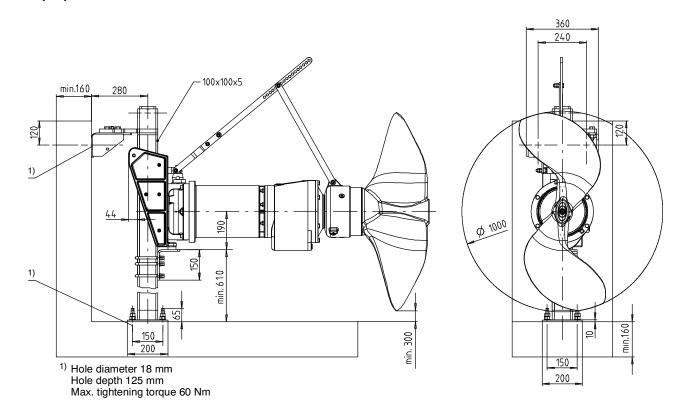
Minimum dimensions for installation through access opening
